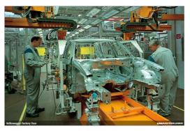
DaimlerChrysler. The laser involved in this new **welding system** does not move from one welding point to the next; instead the **beam of light** is directed at each point using mirrors and beam waveguides. As a result, assembly times should be **reduced** by 90%.
